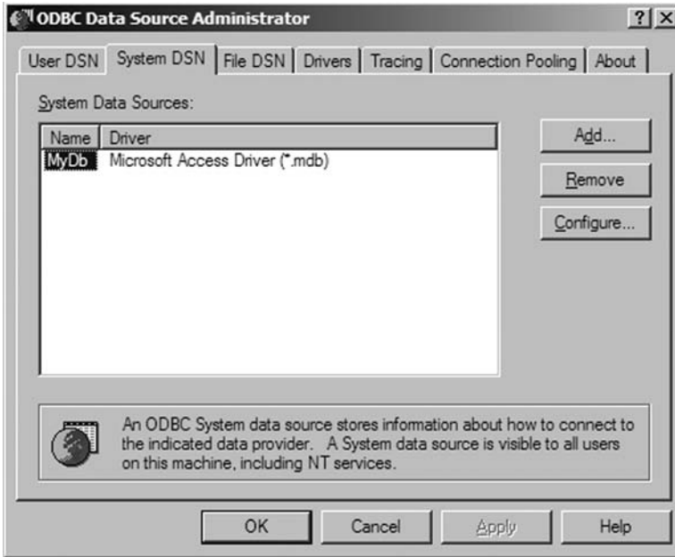
Fig. 2.4 Windows Data Source Administrator with the database MyDb added to the system data source names
