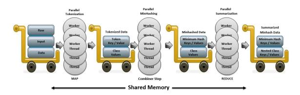
pipeline stages when a locality sensitive hashing engine is deployed.
