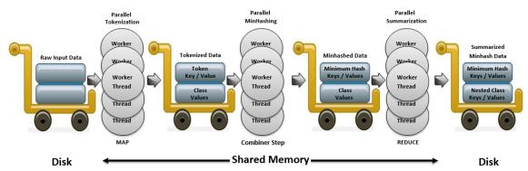
Figure 4.7: Strand Map Reduction Aggregation Processing for a Single Training or Classification Worker Process.
