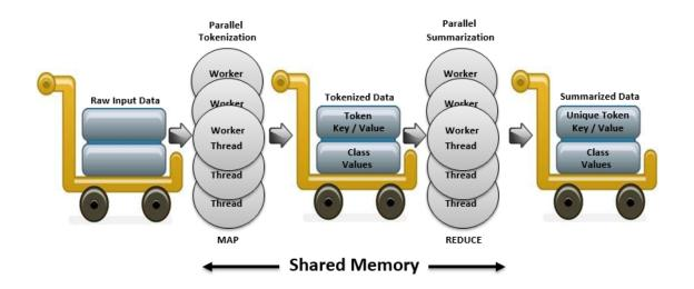
Figure 2.7: Simple Map Reduction Aggregation in the Collaborative Analytics Framework using only a Map and Reduce Stage.
